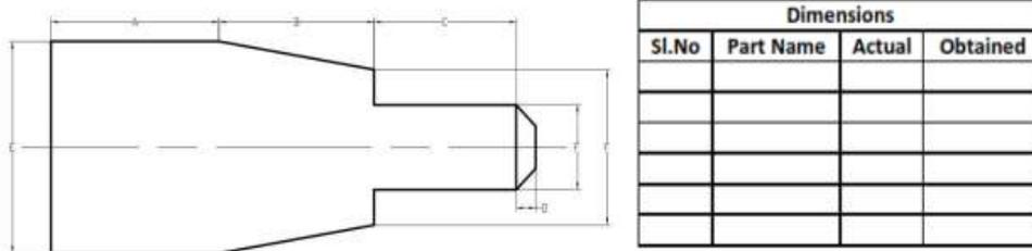
2. Prepare the specimen and make the Step Turing & Thread cutting as shown in figure using the Lathe.
