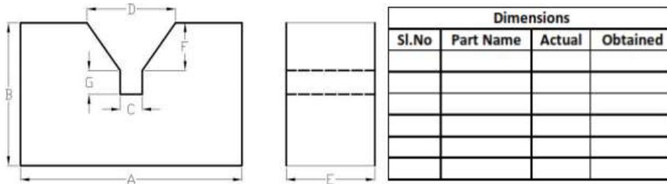
4. Prepare the specimen and make round to square as shown in figure using milling machine
